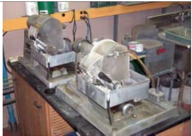
Powders are mixed with epoxy, then spread on a slide and allowed to cure. The surface is ground flat on the thin section grinder, then finished similarly to a thin sections
